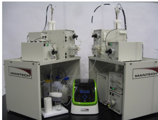
Figure: MANTECH TitraSip SA for automated COD, pH and Alkalinity, Sampling Every 20 Minutes for Effluent Monitoring
